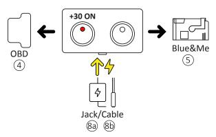
**FIG.2** You can also use the OBD connector (4) as the only power source
